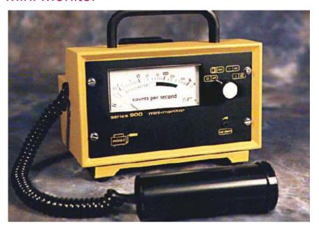
The Mini-monitor serves as a portable or bench top style radiation counter available with a variety of different probes to accommodate most of your radiation detection needs
